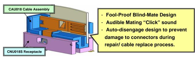
CNU018 Product Series are designed to be the perfect blind-mate FFC connectors. With keyed insulator design for blind-mate function and special auto-disengage function, the product series provides reliable mating quality and durability for product maintenance/replace purposes.
